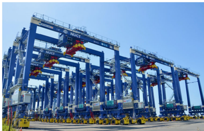
Electric remote-controlled RTGs
