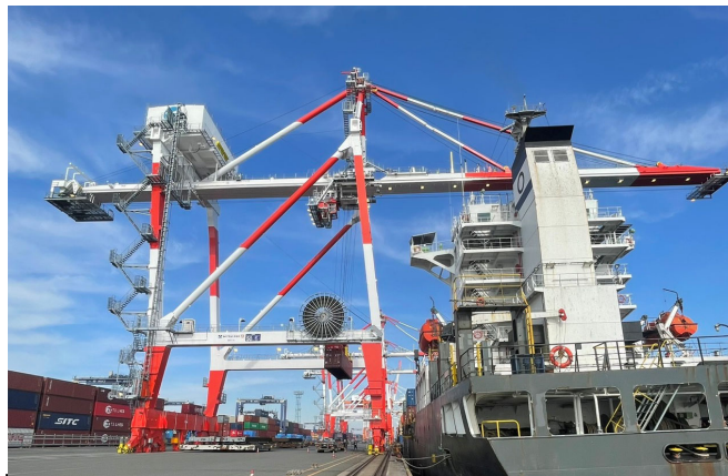
Introduction of inverter-controlled gantry cranes (Newly installed Unit 1)
